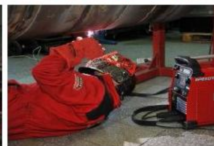
Speedtec 200C: Root pass with TIG DC + FCW SS (Innershield) Fill.
