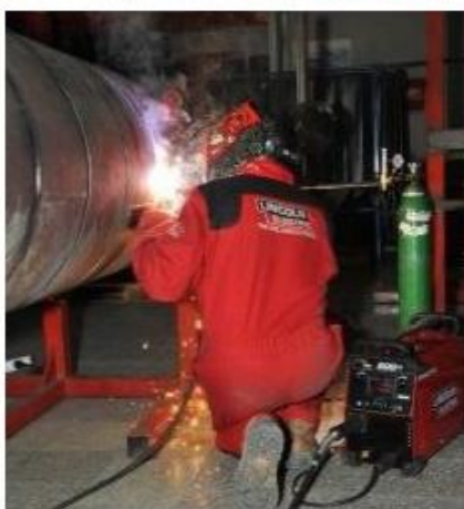
Speedtec 200C: Root pass with TIG DC + FCW SS (Innershield) Fill.
