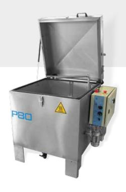
This model is ideal for the automatic washing of small and medium size mechanical parts. The washing is carried out by the action of a series of jets, upper, lower and side, together with the slow motorised rotation of the basket. The operator can program the liquid temperature as well as the length of the treatment cycle.
