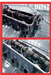
A line of machines for the automatic washing of medium and large size mechanical parts. The high quality of the washing is obtained by special jets and the slow controlled rotation of the basket.
