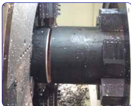
Double hydraulic clamping system font and rear of cut
